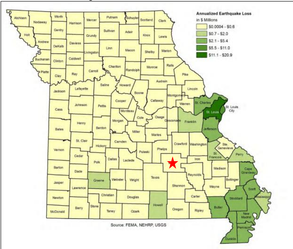
Figure 3.21. HAZUS-MH Earthquake Loss Estimation: Annualized Loss Scenario –Direct Economic Losses to Buildings.
